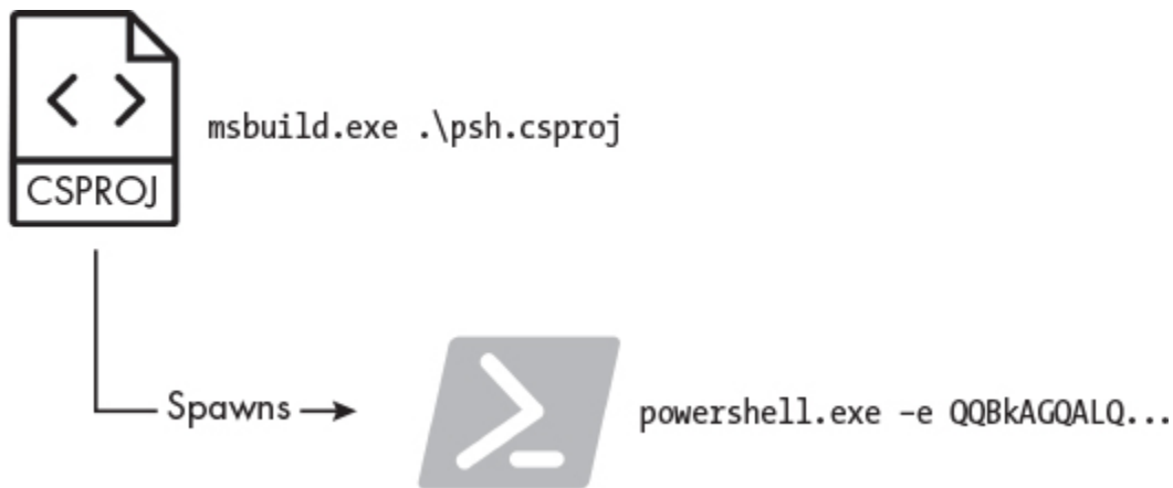
Figure 8-5: The parent-child relationship between MSBuild and an encoded PowerShell command
