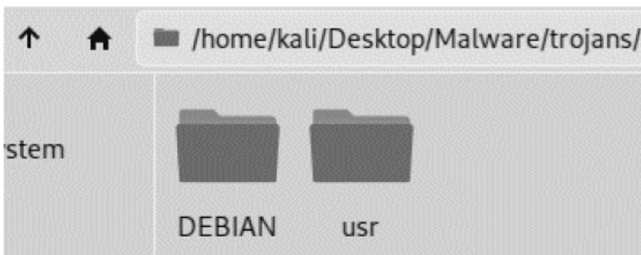
Figure 10-2: The files in the trojans/mailTrojan folder contain the extracted .deb file.
