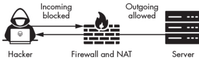
Figure 4-4: How firewalls and NAT block incoming connection, but not outgoing ones
